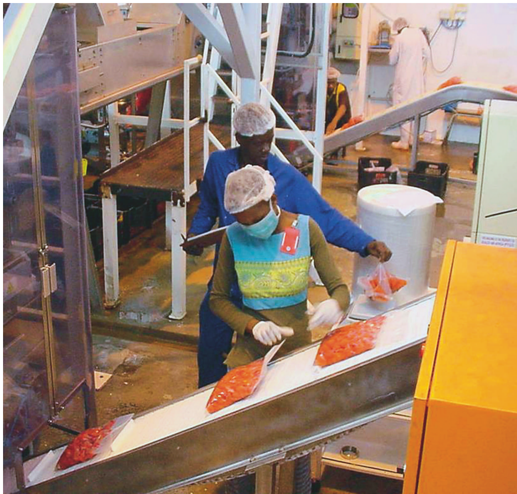
A turnkey vertical pouch-packaging system comprises a product infeed pump for the pepper brine and a bucket conveyor and scales that lead the peppers to a vf/f/s system generating 2-kg foodservice packs.
