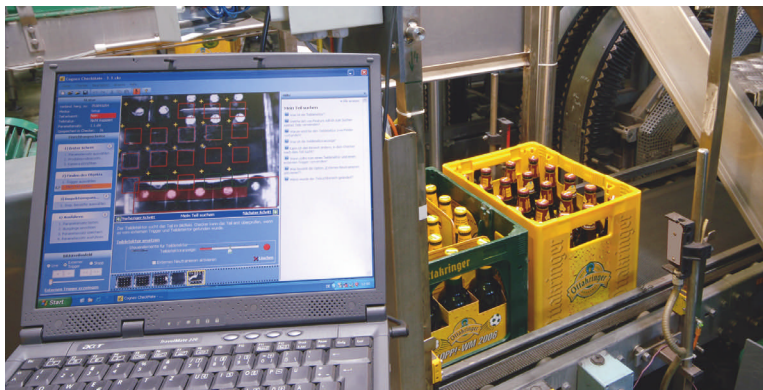
Integrating the sensor into the control technology of Ottakringer's production system was easy due to a standardized interface.
