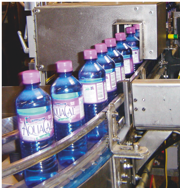
Under a light-controlling hood, out of sight, the sensor inspects fluid-fill levels, left, and tamper-evident safety rings as bottles pass through the inspection station. While this cap, above, looks fine, a tiny gap is found on the left between the cap and the TE ring, a fault detected by the sensor.
