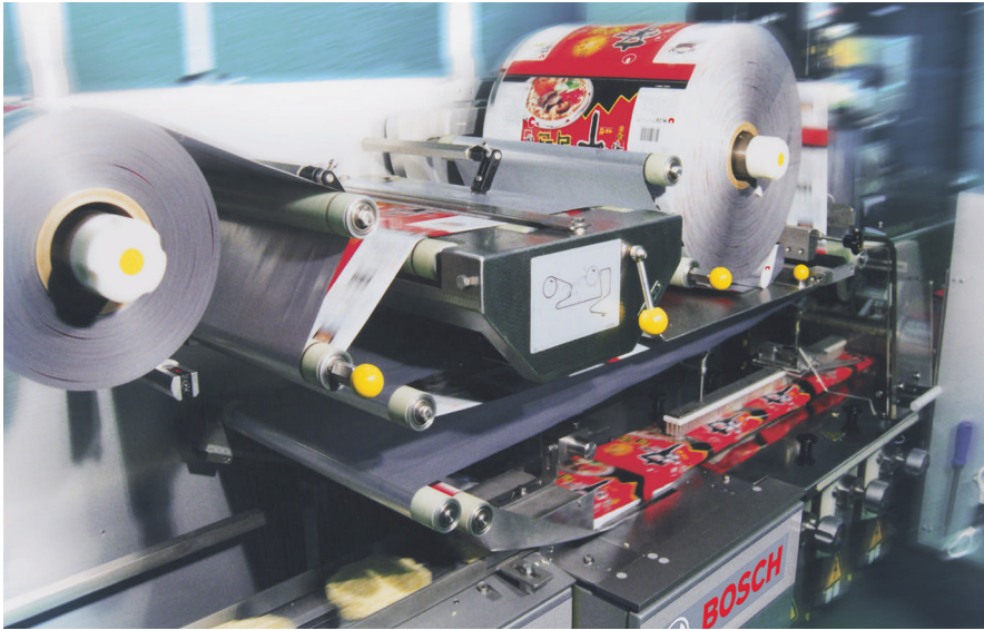
The noodles and sachets are packed by two flowrapper pillow-pack machines producing a total of up to 640 heat-sealed, OPP packs/min.
