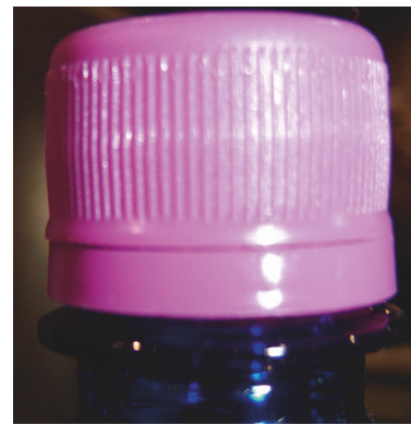
Under a light-controlling hood, out of sight, the sensor inspects fluid-fill levels, left, and tamper-evident safety rings as bottles pass through the inspection station. While this cap, above, looks fine, a tiny gap is found on the left between the cap and the TE ring, a fault detected by the sensor.
